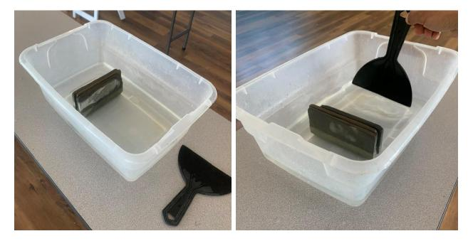
Using the placement of the heavy blockade materials and the putty knife to create waves, show reflection and refraction of waves. Show how groins, jetties, and breakwaters affect these patterns.
